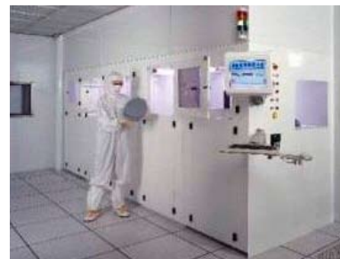
A typical sterile environment of built-in "wet-bench" for wafer rinsing
