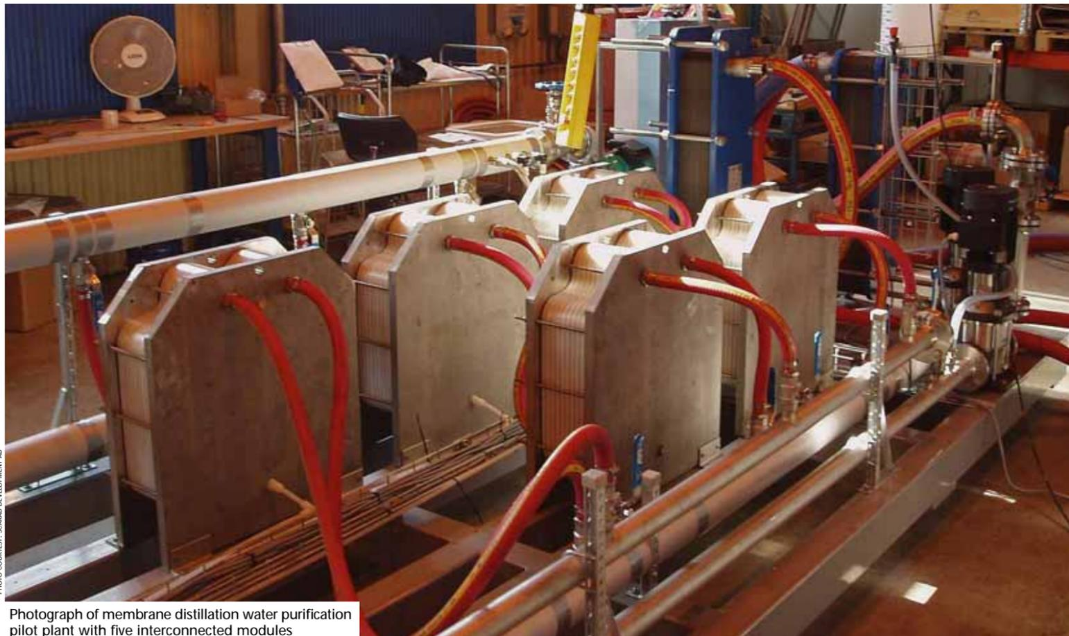
Photograph of membrane distillation water purification pilot plant with five interconnected modules
