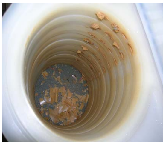
Figure 4. Scale formation at the cassette entrances
