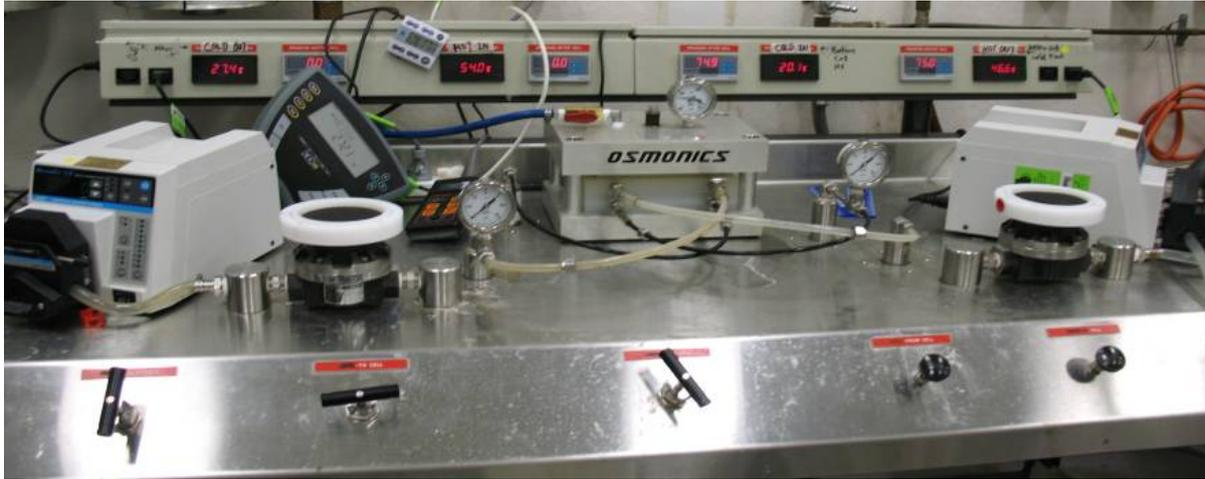
Figure 4 MD apparatus with 0.014 m<sup>2</sup> flat sheet module installed
